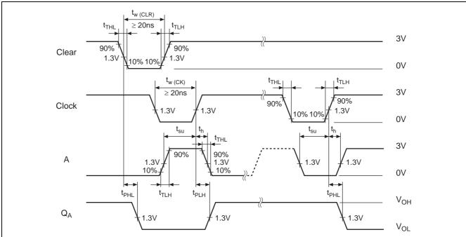
Notes: 1. Input pulse;  $t_{TLH} \le 15$  ns,  $t_{THL} \le 6$  ns, PRR = 1 MHz, (Clock, Clear), PRR = 500 kHz (A or B)
