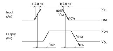
Figure 2 t<sub>pLH</sub>, t<sub>pHL</sub>
