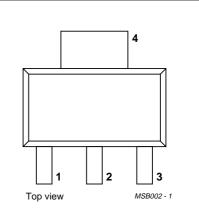
Fig.1 Simplified outline (SOT223) and pin configuration.
