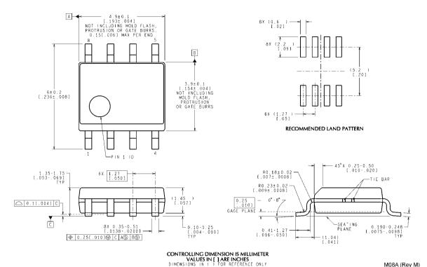
8-Pin SOIC **NS Package Number M08A**  M08A (Rev M)
