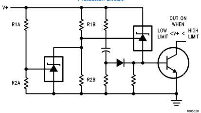
$$\begin{split} & \text{LOW LIMIT} \approx \text{V}_{\text{REF}} \left( 1 + \frac{\text{R1B}}{\text{R2B}} \right) + \text{V}_{\text{BE}} \\ & \text{HIGH LIMIT} \approx \text{V}_{\text{REF}} \left( 1 + \frac{\text{R1A}}{\text{R2A}} \right) \end{split}$$
