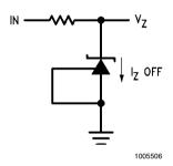
FIGURE 3. Test Circuit for Off-State Current
