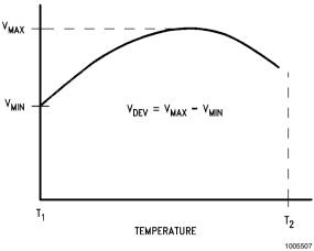
The average temperature coefficient of the reference input voltage,  $V_{REF}$ , is defined as:
