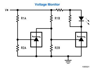
$$\begin{split} \text{LOW LIMIT} &\approx \text{V}_{\text{REF}} \left( 1 + \frac{\text{R1B}}{\text{R2B}} \right) \quad \begin{array}{l} \text{LED ON WHEN} \\ \text{LOW LIMIT} &< \text{V}^+ &< \text{HIGH LIMIT} \\ \end{array} \\ &\text{HIGH LIMIT} &\approx \text{V}_{\text{REF}} \left( 1 + \frac{\text{R1A}}{\text{R2A}} \right) \end{split}$$
