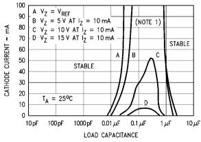
Note: The areas under the curves represent conditions that may cause the device to oscillate. For curves B, C, and D, R2 and V+ were adjusted to establish the initial  $V_Z$  and  $I_Z$  conditions with  $C_L$  = 0.  $V^+$  and  $C_L$  were then adjusted to determine the ranges of stability.
