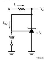
FIGURE 1. Test Circuit for  $V_Z = V_{REF}$
