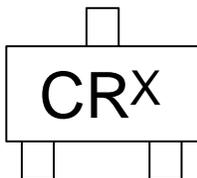
The “X” represents a smaller alpha digit Date Code. The Date Code indicates the actual month in which the part was manufactured.
