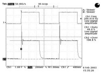
Channel 1 is the Enable waveform to create a change in intensity
