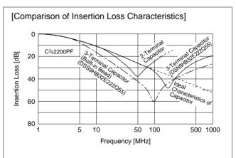
A 3-terminal capacitor has a higher self resonance frequency than a general 2-terminal type and exhibits effective noise suppression at high frequency.
