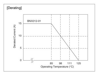
In operating temperatures exceeding +85°C, derating of current is necessary for BNX010 series. Please apply the derating curve shown below according to the operating temperature.
