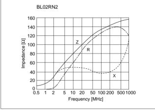
8. Capacitive-Inductive EMI Suppression Filters If capacitive and inductive suppression characteristics are combined, it is possible to configure a much higher performance filter. In signal circuit applications where this combination is applied, noise suppression effects which have little influence on the signal wave form become possible.
