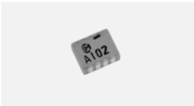
This delay line has been developed by utilizing advanced multilayer technology. It is comprised of a copper line and temperature compensated dielectric NPO ( $0 \pm 60\text{ppm}/^\circ\text{C}$ ) and includes a metal shield. This results in a very small device that is compatible with high frequency applications and SMD chip processing.
