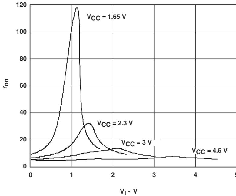
Figure 2. Typical r<sub>on</sub> as a Function of Input Voltage (V<sub>I</sub>) for V<sub>I</sub> = 0 to V<sub>CC</sub>
