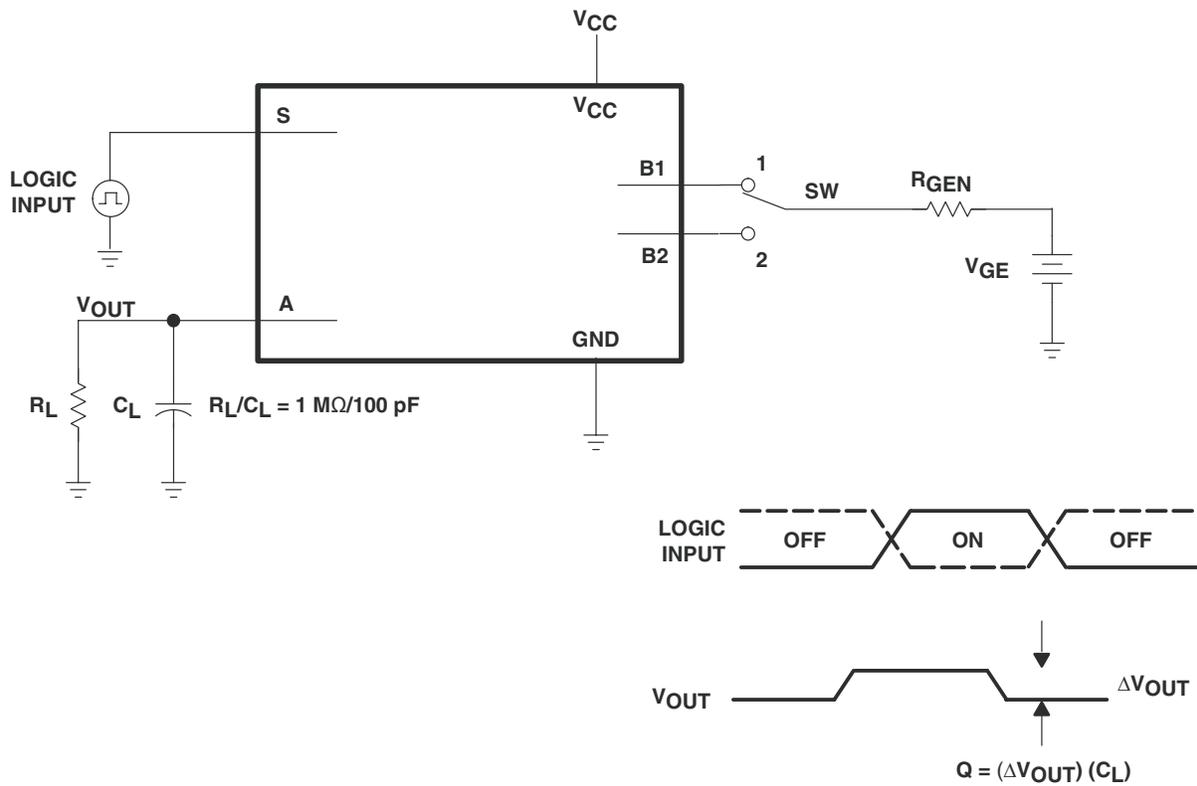
Figure 9. Charge-Injection Test
