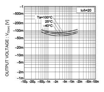
Fig.5 Output voltage vs. output current
