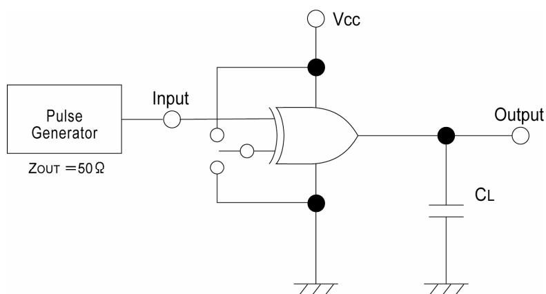
Note: Open output when measuring supply current
