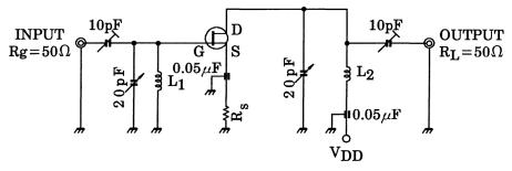
$L_1{:}~0.8~\text{mm}\phi~A_g$  plated Cu wire, 3 turns, 10 mm ID, 10 mm length.
