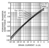
Fig.8 Forward transfer admittance vs. drain current
