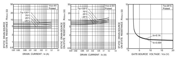
Fig.4 Static drain-source on-state resistance vs. drain current (I)
