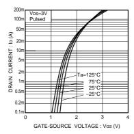
Fig.2 Typical transfer characteristics
