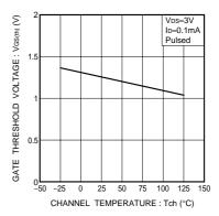
Fig.3 Gate threshold voltage vs. channel temperature
