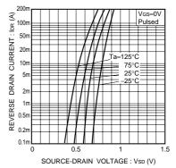
Fig.9 Reverse drain current vs. source-drain voltage (I)
