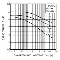
Fig.11 Typical capacitance vs. drain-source voltage
