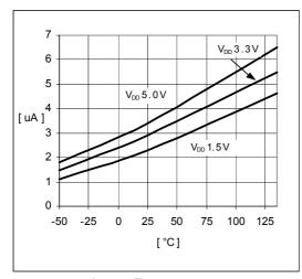
I<sub>DD</sub> vs. Temperature
