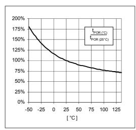
Reset Timeout Period t<sub>POR</sub> vs. Temperature (normalized with respect to t<sub>POR 25°C</sub>)
