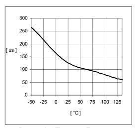
Propagation Time t<sub>P</sub> vs. Temperature
