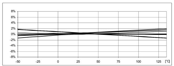
Threshold Voltage Variation vs. Temperature (normalized)
