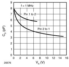
Figure 3. Typical Capacitance  $C_D$  vs. Reverse Voltage  $V_B$
