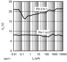
Figure 4. Typical Reverse Voltage  $V_{\mbox{\scriptsize R}}$  vs. Reverse Current  $I_{\mbox{\scriptsize R}}$
