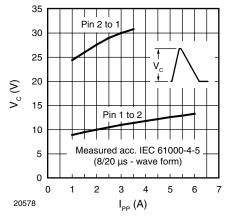
Figure 5. Typical Peak Clamping Voltage  $V_{\rm C}$  vs. Peak Pulse Current  $I_{\rm PP}$
