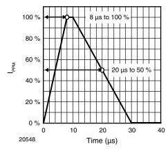
Figure 1. 8/20 µs Peak Pulse Current Wave Form (acc. IEC 61000-4-5)
