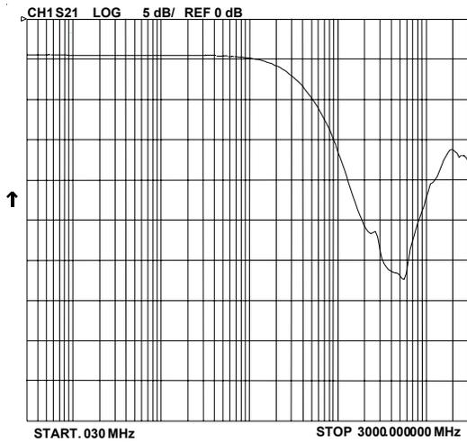
Typical Insertion loss (A3-B3 to Gnd)
