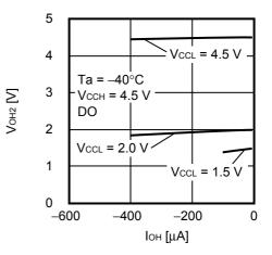
1. 25 High level output voltage V<sub>OH2</sub> vs. High level output current I<sub>OH</sub>
