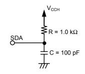
Figure 7 Output Load Circuit
