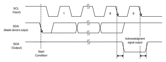
Figure 23 Acknowledgment Output Timing 1
