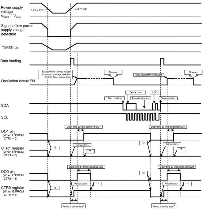
\*1. The value of control port register does not change even if the port output is inverted by timer action.
