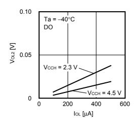
1. 23 Low level output voltage V<sub>OL2</sub> vs. Low level output current I<sub>OL</sub>
