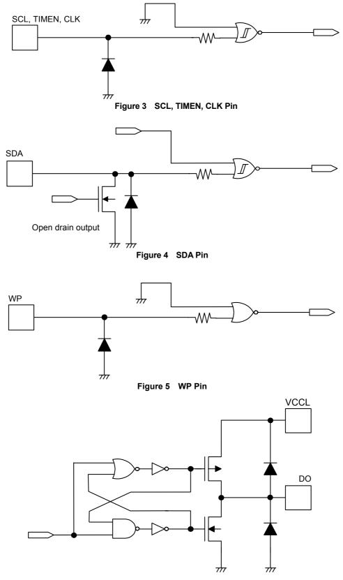
Figure 6 DO Pin and VCCL Pin
