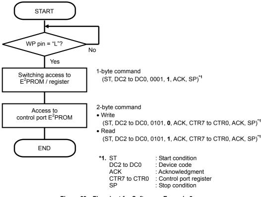
Figure 29 Flowchart for Software Example 2
