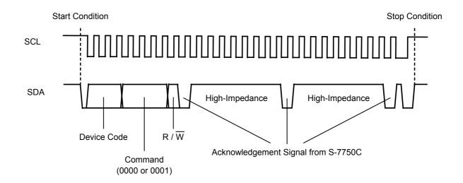
Figure 24 Acknowledgment Output Timing 2
