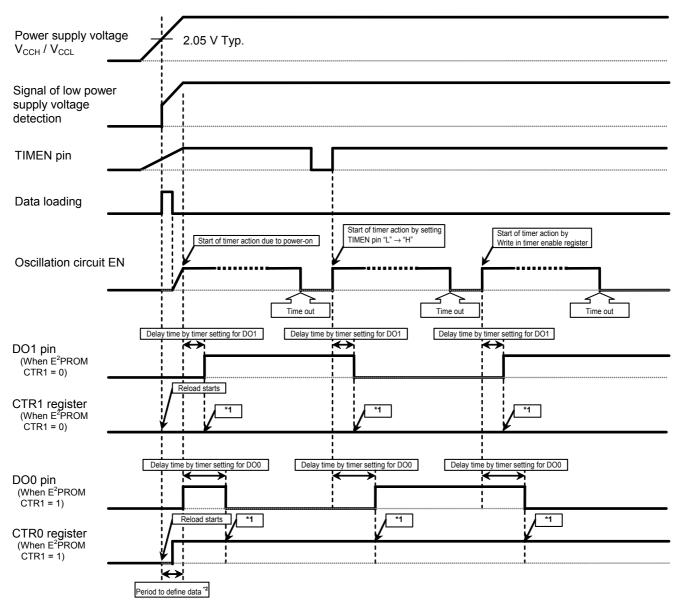
\*1. The value of control port register does not change even if the port output is inverted by timer action.
