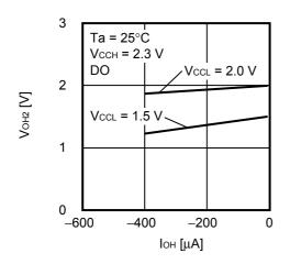
1. 29 High level output voltage V<sub>OH2</sub> vs. High level output current I<sub>OH</sub>
