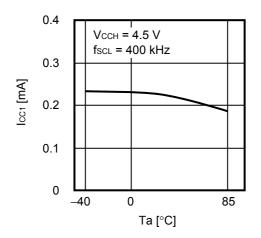
1.3 Current consumption (READ) I<sub>CC1</sub> vs. Ambient temperature Ta
