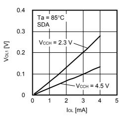
1.22 Low level output voltage  $V_{OL2}$ vs. Low level output current  $I_{OL}$
