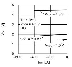
1.28 High level output voltage V<sub>OH2</sub> vs. High level output current I<sub>OH</sub>
