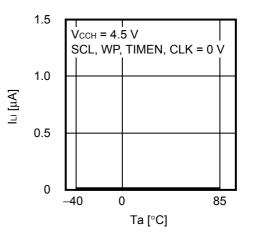
1.16 Output leakage current I<sub>LO</sub> vs. Ambient temperature Ta
