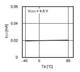
1. 11 Internal oscillator current consumption during operation Icc3 1. 12 Internal oscillator current consumption during operation Icc3 vs. Ambient temperature Ta
