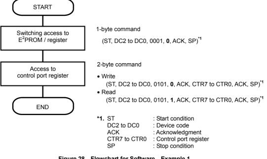
Figure 28 Flowchart for Software Example 1
