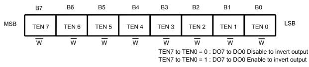
Figure 11 Timer Enable Register
