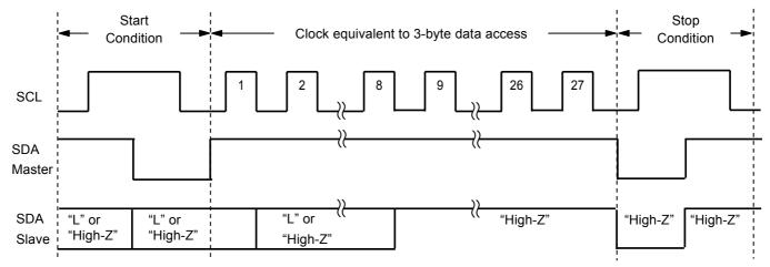
Figure 31 How to Reset S-7750C
