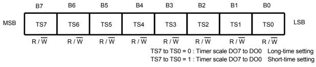
Figure 13 Timer Scale Setting Register / E<sup>2</sup>PROM
