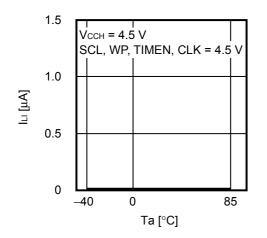
1. 17 Output leakage current I<sub>LO</sub> vs. Ambient temperature Ta
