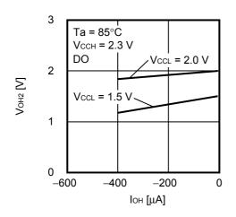
1.26 High level output voltage V<sub>OH2</sub> vs. High level output current I<sub>OH</sub>
