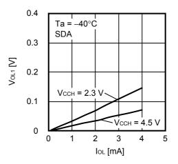
1. 19 Low level output voltage V<sub>OL1</sub> vs. Low level output current I<sub>OL</sub>
