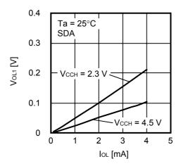
1. 21 Low level output voltage V<sub>OL2</sub> vs. Low level output current I<sub>OL</sub>
