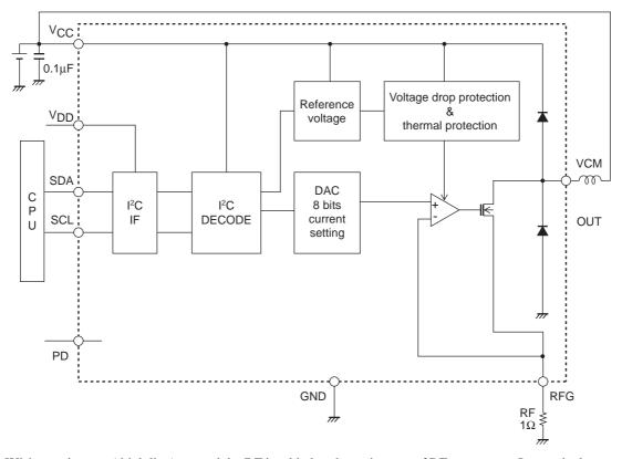
Wiring resistance (thick line) around the RF is added to the resistance of RF as an error. It must be kept as small as possible.
