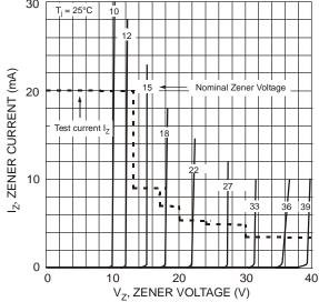
Fig. 3 Typical Zener Breakdown Characteristics
