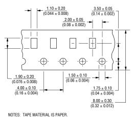
TAPE MATERIAL IS PAPER. TAPE THICKNESS IS  $\frac{0.60 \pm 0.05}{(0.024 \pm 0.002)}$  COVER TAPE ADHESION IS 40 ± 15 GRAMS.
