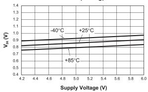
V<sub>IL</sub> vs. Supply Voltage EN Pin (Falling)
