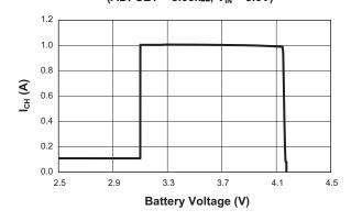
Fast Charge Current vs. Supply Voltage (ADPSET = 8.06kΩ)
