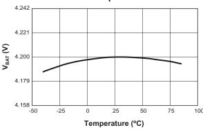
Preconditioning Threshold Voltage vs. Temperature
