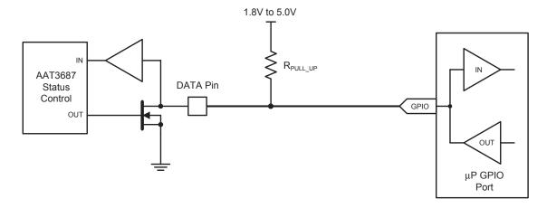
Figure 3: Data Pin Application Circuit.
