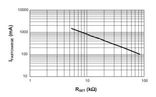
Figure 2: I<sub>FASTCHARGE</sub> vs. R<sub>SET</sub>.
