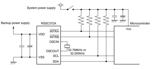
\*) The SCL and SDA pins of the RS5C372A do not contain protective diodes on VDD side. Therefore, back up power supply system power supply causes no adverse effect.
