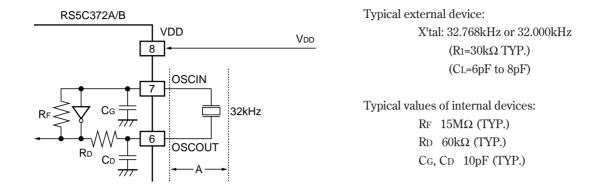
The oscillation circuit is driven at a constant voltage of about 1.2V relative to the Vss level.
