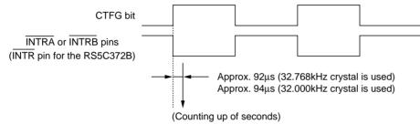
\*) Since counting up of seconds and the falling edge has a time lag of approx. 92µs (at 32.768kHz) (approx. 94µs when 32.000kHz crystal is used), a time may be read with apparently approx. one second delayed from time of the real-time clock when time is read in synchronization with the falling edge of output.
