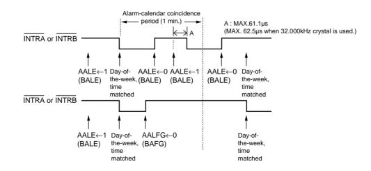
\*) Note that AAFG (BAFG) has an output wave form of reversed logic.
