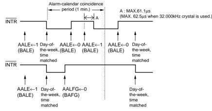
\*) Note that AAFG (BAFG) has an output wave form of reversed logic.
