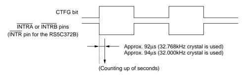
\*) Since counting up of seconds and the falling edge has a time lag of approx. 92µs (at 32.768kHz) (approx. 94µs when 32.000kHz crystal is used), time with apparently approx. one second of delay from time of the real-time clock may be read when time is read in synchronization with the falling edge of output.
