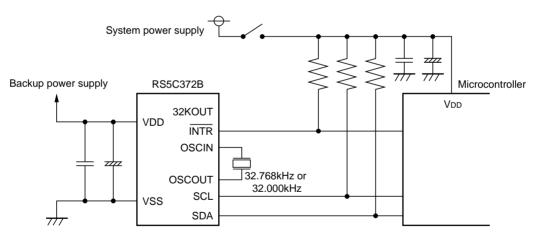
\*) The SCL and SDA pins of the RS5C372B do not contain protective diodes on VDD side. Therefore, back up power supply system power supply causes no adverse effect.
