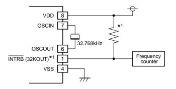
X'tal: 32.768kHz (R1=30kΩ TYP.) (CL=6pF to 8pF) Topt: 25°C Output pins : Open
