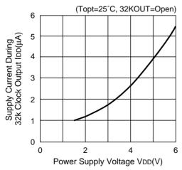
vs. Power Spply Voltage (RS5C372A)
