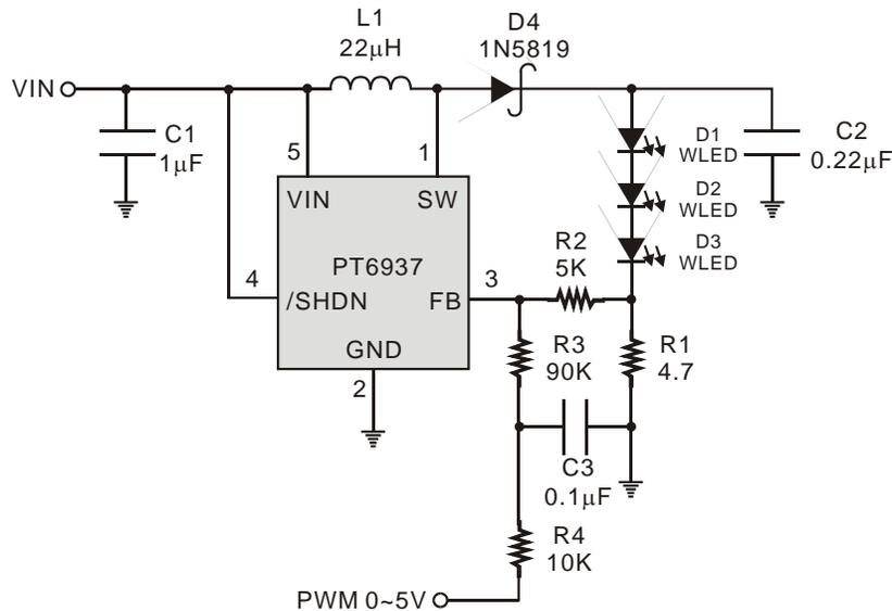
Figure 4. Dimming Control Using Filtered PWM Signal.
