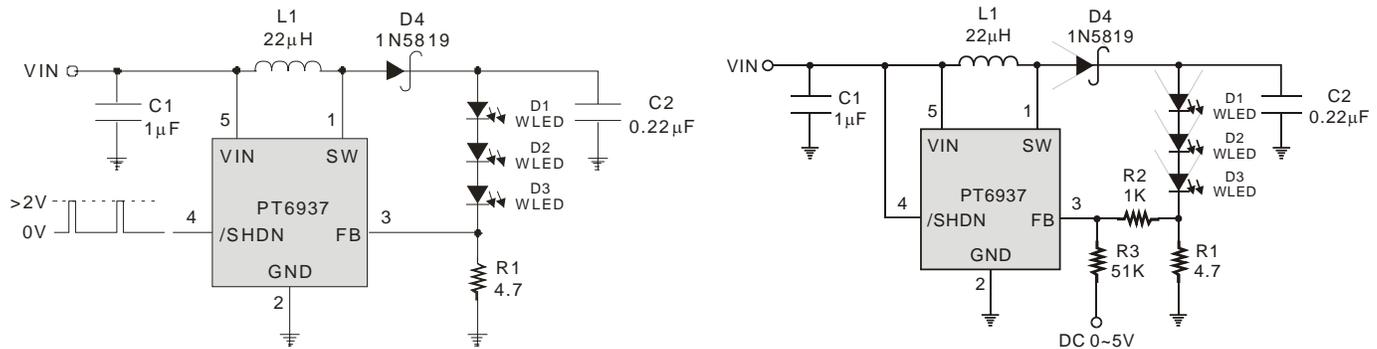
Figure 2. PWM Dimming control Using the /SHDN Pin      Figure 3. Dimming Control Using DC Voltage
