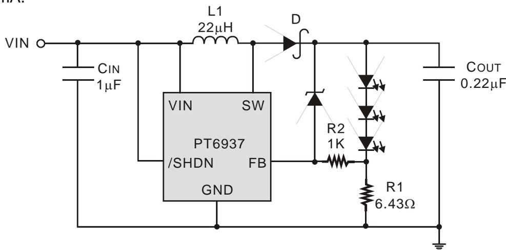
Figure1. LED driver with open-circuit protection
