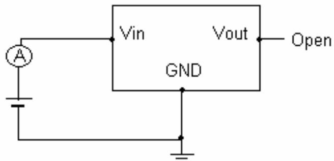
**Measuring Circuit 2: Output Voltage, Oscillation Check, Line Regulation, Dropout Voltage, Load Regulation**
