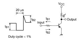
Figure 1 Switching Time Test Circuit & Timing Chart
