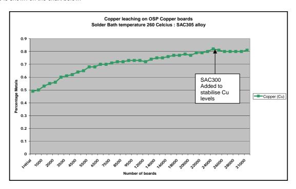
This shows an average leaching rate of **0.01% Cu per 1000 boards**. Each process is unique this is an indication only of the leaching rate (based on actual data).
