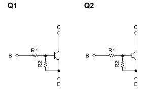
1.6±0.05 1.2±0.05 6 0.2±0.05 0.5 1.6±0.05 0.0±0.05 5 0.5 05 0.55±0.0 0.12±0.05 1. EMITTER 1 2. BASE 1 3. COLLECTOR 2 (E1) (B1)(C2)4. EMITTER 2 (E2) 5. BASE 2 6. COLLECTOR 1 (B2) (C1) ES6 JEDEC \_ JEITA TOSHIBA 2-2N1G
