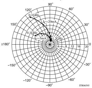
$\begin{array}{l} S22e: V_{CE}\!\!=\!\!10V \\ f\!\!=\!\!100MHz, 200 \text{ to } 1200MHz (200MHz \text{ step}) \end{array}$
