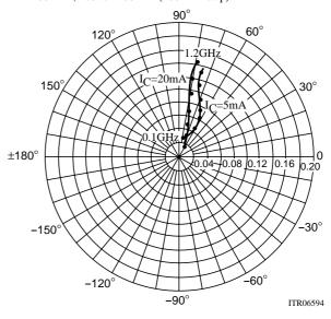
$\begin{array}{l} S21e:V_{CE}{=}10V\\ f{=}100MHz,\,200\;to\;1200MHz(200MHz\;step) \end{array}$
